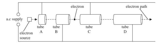
(i) An electron is shown between tubes B and C.
